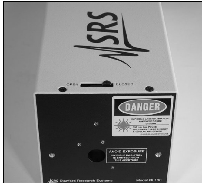
Figure 13. Front of the NL100 laser system, showing the beam shutter in the closed position.
