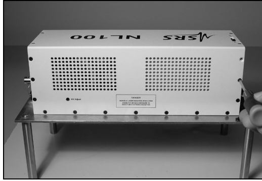
Figure 16. Remove the screws on the protective housing.
