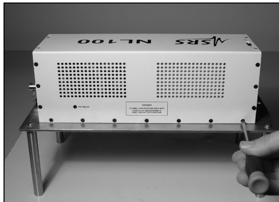
Figure 24. Secure protective cover with Phillips screws.
