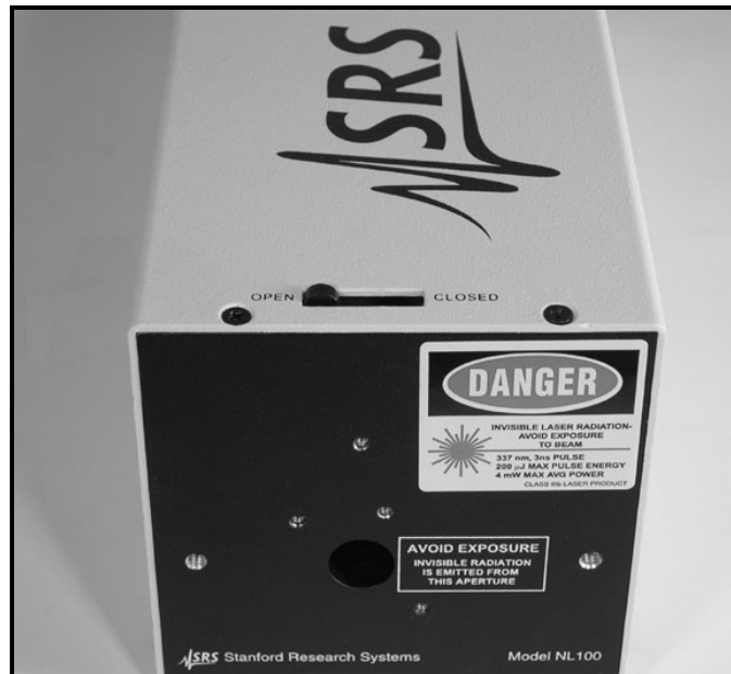
Figure 14. Front of the NL100 laser system, showing the beam shutter in the open position.
